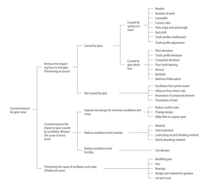
Fig. 1 Cause and solution for gear noise
